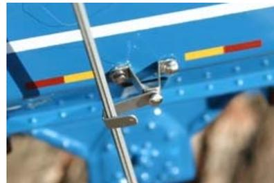
Studs are included for the axle assemblies on the row crop models. Glue these in place as shown, on both front and rear.
